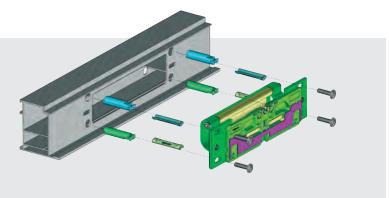
Application with clamping achors. (Also possible with clamping plates.)
